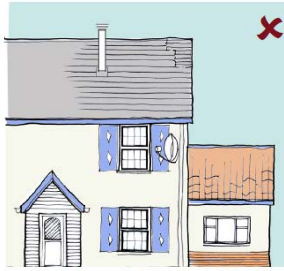
Example 2: Unsympathetic repairs and alterations
