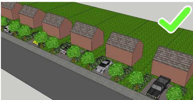
6.22 In the case of narrow fronted dwellings (typically 5m wide) the frontage parking must not take up more than half the width of the individual plots and must not obstruct access for all to the front door.
