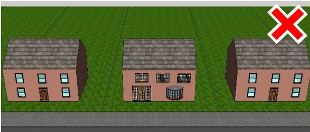
6.16 Where a traditional pitched roof is proposed, this should generally match the pitch and orientation of existing roofs to either side.
