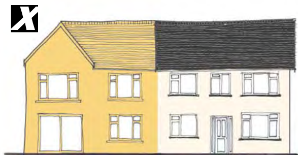
FIGURE 19: A poorly designed side extension that competes with the scale and form of the original house
