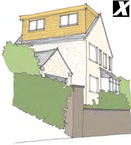
FIGURE 32: A large, poorly designed dormer extension can dominate a house and the streetscene
