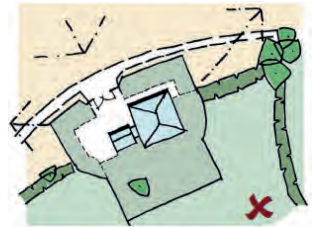
Below: Insensitive location of the buildings, removal of hedgerows and creation of garden to front detracts from the long views
