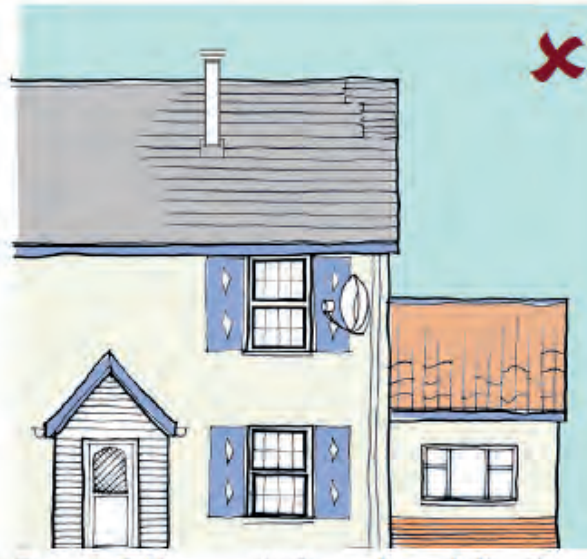
Example 2: Unsympathetic repairs and alterations
