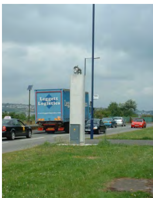
Figure 2.1.1.5 - St Thomas DOAS Transmitter
