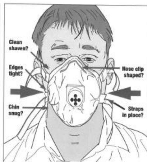
7 Before entering the workplace, a user seal check should be carried out. This is done by placing your hands over the filter material and breathing in. The mask should suck down onto your face when you breathe in sharply. You should hold your breath for ten seconds and the disposable respirator should not loosen. If it does, you should readjust and repeat.
